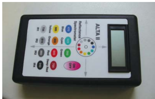
Figure 3: ALTA II portable on-field spectrophotometer
