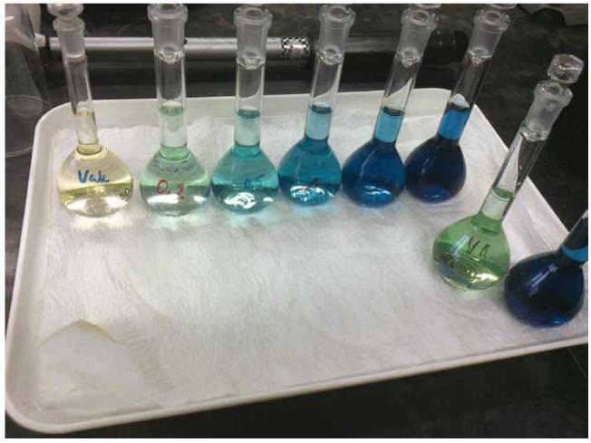
Figure 2: Some water samples for NH<sub>4</sub><sup>+</sup> analysis via photometric method
