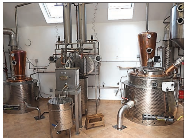
Figure 5: Pot-still double-distillation apparatus – Veresi Pálinkaház, Vere-segyház
