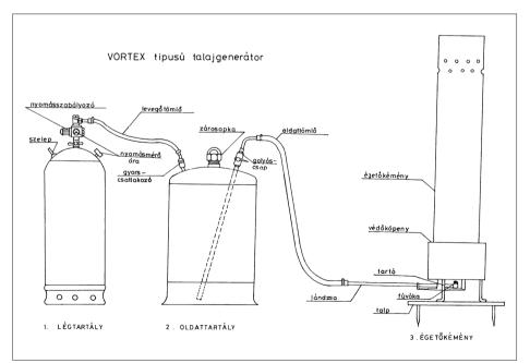
Figure 2: Main units of the soil generator used by NEFELA: air tank (1), solution tank (2) and incinerator (3)
