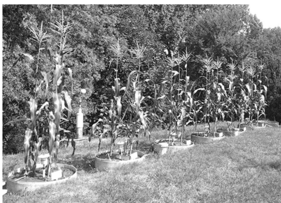
Figure 1. Dessert R78 F 1 sweet corn grown in the simple drainage lysimeters (Karcag, 2019)
